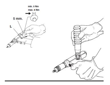
IMPORTANT: Make sure plug (L) is tightened at a torque corresponding to min. of 3.6 ft-lb and a max. Of 5.9 ft-lb
